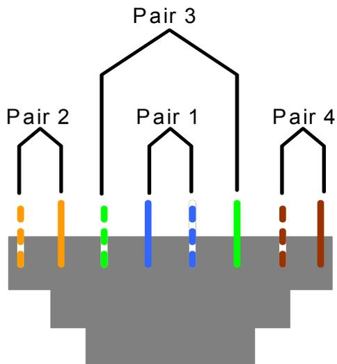
Figure 9 T568B Wiring
