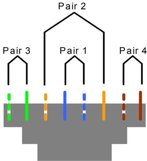
Figure 8 T568A Wiring
